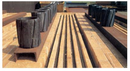
Automatic operation means overnight treatments can be programmed unattended at reduced tariffs. This, coupled with the low thermal mass insulation gives rapid heat up and low energy costs.
